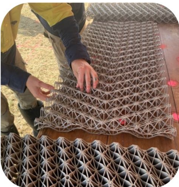
Assembly of BESE-Elements® (Photo – Angus Frazer)
